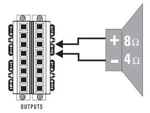
Stereo or parallel connection- single speaker shown connected to amplifier channel 6 output. Ensure that all speaker connections maintain proper polarity ( + to +, - to - ).
